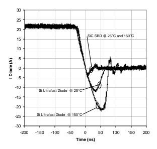
Figure 6: 600 volt turn off current of the Si Ultrafast diode and the SiC SBD at 25°C and 150°C.
