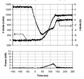
Figure 10. 1200 volt Si Ultrafast diode turnoff voltage, current and instantaneous power at 125°C.
