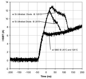
Figure 15: 1200 volt turn-on current of the IGBT w/ the Si Ultrafast diode and the SiC SBD at 25°C and 150°C.
