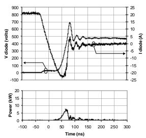
Figure 2. 600 volt Si Ultrafast diode turn-off voltage, current and instantaneous power at 150°C.
